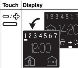
The information for a saved heating phase of the active weekly program is shown on the display (here: not heating phase stored).
